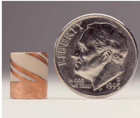
Figure 4. Small PowerHelix Antenna with Center Frequency \approx 2GHz
